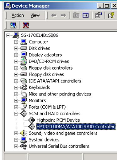
If you cannot find these two device items, or there is ? or ! on device icon, it indicates that the driver has not been correctly installed and needs reinstallation.
