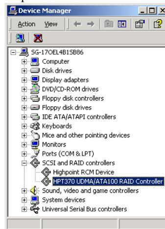
If **HPT370 UDMA/ATA100 RAID Controller** or **HPT372 UDMA/ATA 133 RAID Controller** item exists in the popup **Device Manager** window, it indicates that the driver has been successfully installed. Otherwise, please reinstall the driver.
